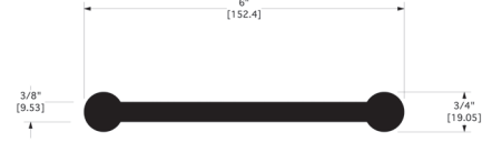
PVC648 6" Dumbbell Waterstop 125 ft Head of H 2 O • 50 lft/roll • 1.59 lbs/lft
