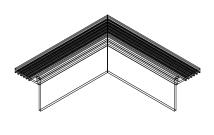
3) Heat weld waterstop profile to appropriate length and directional changes to fit concrete surface.
