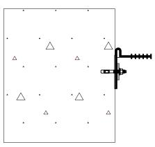
10) Hammer stainless steel wedge anchors into drilled holes, passing anchor through batten bar, waterstop and epoxy gel bed. Repeat for all holes. Tighten anchor bolts.
