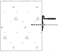
5) Using the prepunched stainless steel batten 6) M bar as a template, drill 1/4" holes 2-3/4" deep per r through waterstop and concrete. Clean out holes. can.
