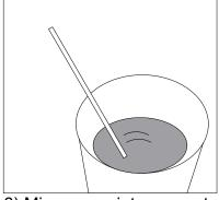
6) Mix appropriate amount of epoxy per mixing instructions on epoxy s. can.
