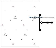
5) Using the prepunched stainless steel batten 6) M bar as a template, drill 1/4" holes 2-3/4" deep per r through waterstop and concrete. Clean out holes. can.
