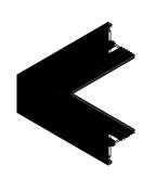
3) Heat weld waterstop profile to appropriate length and directional changes to fit concrete surface.
