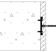
11) If expansion joint install expansion joint filler above and beneath waterstop embedment leg.
