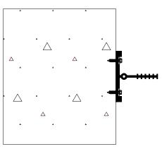
10) Install Tapcons into drilled holes, passing anchor through batten bar, waterstop and epoxy gel bed. Repeat for all holes. Tighten all the fasteners.
