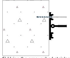
5) Using the prepunched stainless steel batten 6) M bar as a template, drill 1/4" holes 2-3/4" deep per r through waterstop and concrete. Clean out holes. can.
