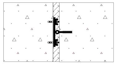
12) Allow installed retrofit waterstop system to cure for 24 hours before placing the second pour of concrete.
