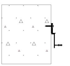
10) Install Tapcons into drilled holes, passing anchor through batten bar, waterstop and epoxy gel bed. Repeat for all holes. Tighten all the fasteners.
